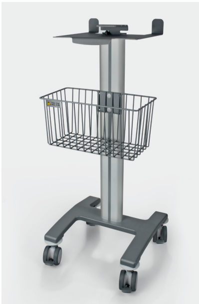
Mobile Stand with Basket / 4 castors with castor lock (2 include ESD), height 939 mm (37"), width 400 mm (16"), depth 400 mm (16"), 8.2 kg (18.1 lbs)
